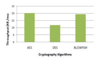
Figure 2: Throughput of Audio Files Decryption
